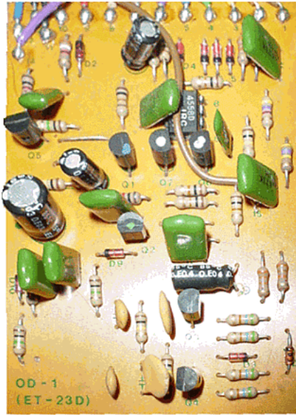
Fig. 2: Boss OD-1 OverDrive circuit board - component side (ET-23D version)
